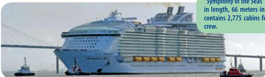
"Symphony of the Seas" is a floating resort town, 72 meters in depth, 362 meters in length, 66 meters in width, with the deadweight of 230,000 tons. A vessel contains 2,775 cabins for 6,780 passengers, serviced by 2,175 members of the crew.
